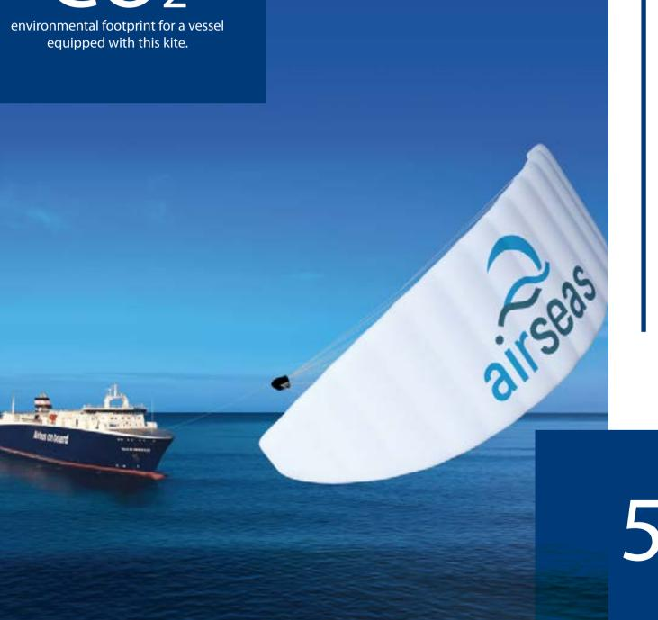
Seawing is an automated kite based on parafoil technology, used to tow commercial vessels. Seawing also analyzes a large quantity of complex data in real time and autonomously adapts to current conditions to optimize the vessel's performance while guaranteeing maximum safety. The expected fuel savings will reduce the CO2 environmental footprint for a vessel equipped with this kite.
